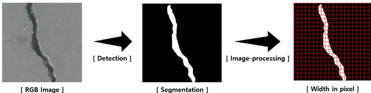
**Fig. 1** Overview of crack quantification
